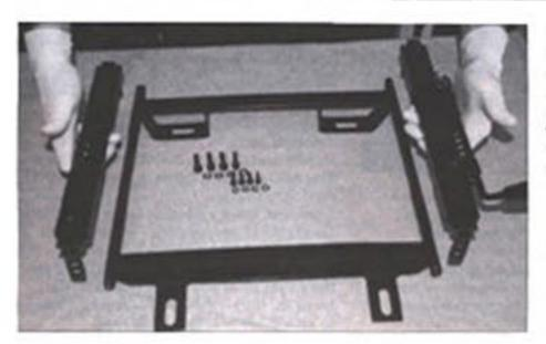
1 The other bracketry option is to use what Seat Source supplies for the Mustang. This three-piece manual setup is much simpler than the factory manual rack and weighs a lew pounds loss, but does essentially the same thing.
